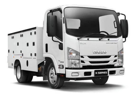
Fully powdercoated steel service body / 7 lockable storage compartments with a total volume of 2.5 cubic metres / 2.08 m x 1.0 m (L x W) central storage area with chequerplate floor and 6 tie down points / 2,500 kg rated towbar with integrated rear step / Storage compartment locking integrated with vehicle central locking system / LED lighting in each storage compartment / Rear barn door for central storage area / Rear grab handles and non slip step surfaces / Isuzu reversing camera
