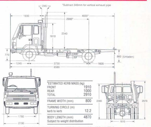
\*Chassis and cab with oil, water and fuel tank containing 10 litres of fuel.
