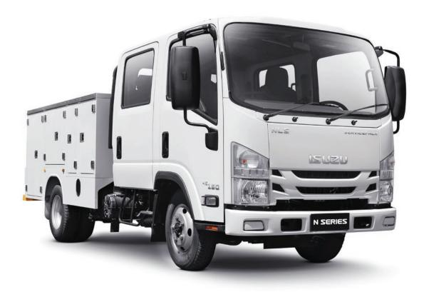
Fully powdercoated steel service body / 7 lockable storage compartments with a total volume of 3.2 cubic metres / 1.88m x 1.0m (L x W) central storage area with chequerplate floor and 4 tie down points / Storage compartment locking integrated with vehicle central locking system / LED lighting in each storage compartment / Rear barn door for central storage area / Rear grab handles and non slip step surfaces / 2,500kg rated towbar with integrated rear step / Isuzu reversing camera
