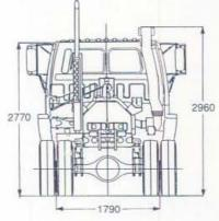
\*Chassis and cab with oil, water and fuel tank containing 10 litres of fuel. \*15,000 kg off road 18,000 kg on road
