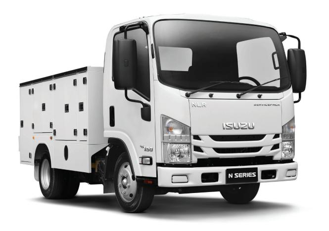
Fully powdercoated steel service body / 7 lockable storage compartments with a total volume of 2.9 cubic metres / 2.08 m x 1.0 m (L x W) central storage area with chequerplate floor and 6 tie down points / 2,500 kg rated towbar with integrated rear step / Storage compartment locking integrated with vehicle central locking system / LED lighting in each storage compartment / Rear barn door for central storage area / Rear grab handles and non slip step surfaces / Isuzu reversing camera
