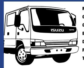
Model NPR250/300 Crew Cab GVM 4,490kg/6,200kg GCM 7,990kg/9,700kg **Engine Type: Isuzu SiTEC 115** Displacement: 4,570 cc 85 kW @ 3,200 RPM Power\*: 291 Nm @ 1,600 RPM Torque\*:
