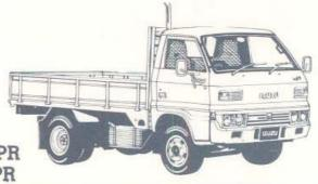
TLD 24 GVM 4200kg; GCM 6300kg with 7.50 x 15 - 10 PR TLD 44 GVM 4800kg; GCM 6300kg with 7.50 x 15 - 8 PR
