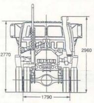
"Chassis and cab with oil, water and fuel tank containing 10 litres of fuel. \*15,000kg off road 18,000kg on road.
