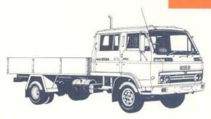
GVM  $8000 \text{ kg} (17,637 \text{ lb}) \text{ with } 8.25 \times 16 - 12 \text{ ply tyres.}$
