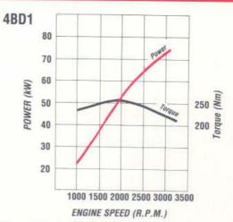
Type: 4 Cylinder OHV diesel ■ Bore x Stroke (mm) 102 x 118 ■ Displacement 3856 (cc) ■ Compression ratios (:1) 17.0 ■ Output-Power (kW) 76 @ 3200 rpm (DIN Nett) ■ Torque (Nm) 255 @ 1900 rpm (DIN Nett)
