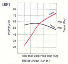
Type: 4 Cylinder direct injection diesel ■ Bore x Stroke (mm) 105 x 105 ■ Displacement 3636 (cc) ■ Compression ratios (:1) 17.5 ■ Output-Power (kW) 74 @ 3500 rpm (DIN Nett) ■ Torque (Nm) 242 @ 2000 rpm (DIN Nett)
