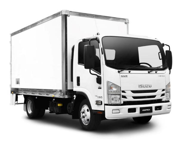
4.27m(L) x 2.185m(W) x 2.085(H) van body / Fibreglass honeycomb front, side and rear door panels / Aluminium roof panel / Rear barn doors with camlocks / Internal tie down rails / 200mm high protective aluminium internal kickpanel / Rear grab handles and step / Provision for rear tailgate loader / LED interior lighting / Isuzu satellite navigation and reversing camera
