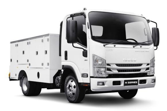
Fully powdercoated steel service body / 7 lockable storage compartments with a total volume of 3.7 cubic metres / 2.28m x 1.17m (L x W) central storage area with chequerplate floor and 6 tie down points / Storage compartment locking integrated with vehicle central locking system / LED lighting in each storage compartment / Rear barn door for central storage area / Rear grab handles and non slip step surfaces / 3,500kg rated towbar with integrated rear step / Isuzu reversing camera
