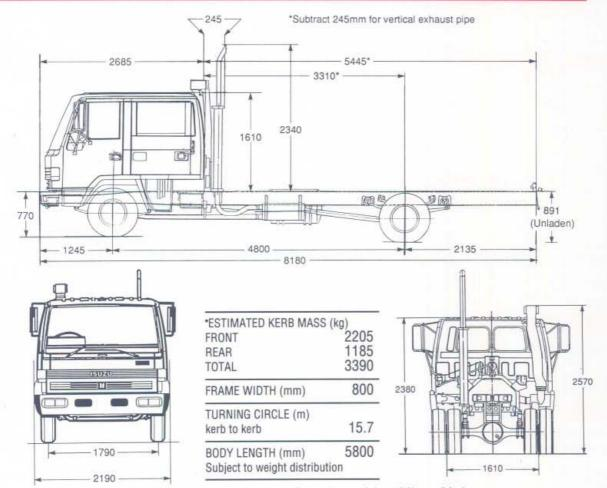
\* Chassis and cab with oil, water and fuel tank containing 10 litres of fuel.
