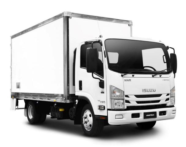
4.27m(L) x 2.185m(W) x 2.085(H) van body / Fibreglass honeycomb front, side and rear door panels / Aluminium roof panel / Rear barn doors with camlocks / Internal tie down rails / 200mm high protective aluminium internal kickpanel / Rear grab handles and step / Provision for rear tailgate loader / LED interior lighting / Isuzu reversing camera
